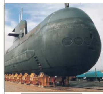
The six torpedo tubes can easily be seen on the front of HMAS Rankin.
