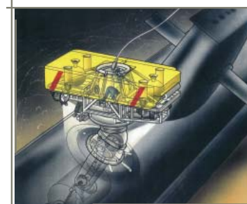
This diagram shows REMORA attached to the escape tower.
