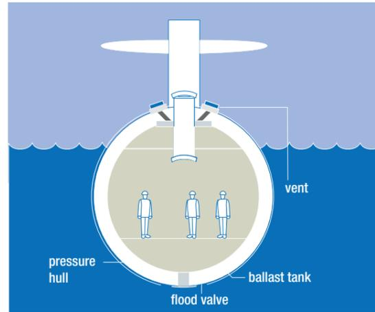
This simplified diagram shows a submarine's ballast tanks filled with air, allowing it to float on the surface. Not all submarines have ballast tanks around the hull. The Collins Class, for example, has ballast tanks located inside the hull.
