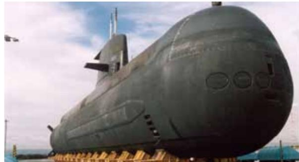
The six torpedo tubes can easily be seen on the front of HMAS Rankin.
