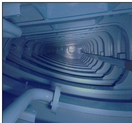
Fig. 10. Tankage implemented with a single coat paint scheme
