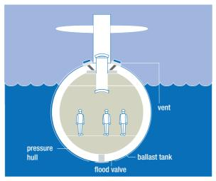
This simplified diagram shows a submarine's ballast tanks filled with air, allowing it to float on the surface. Not all submarines have ballast tanks around the hull.
